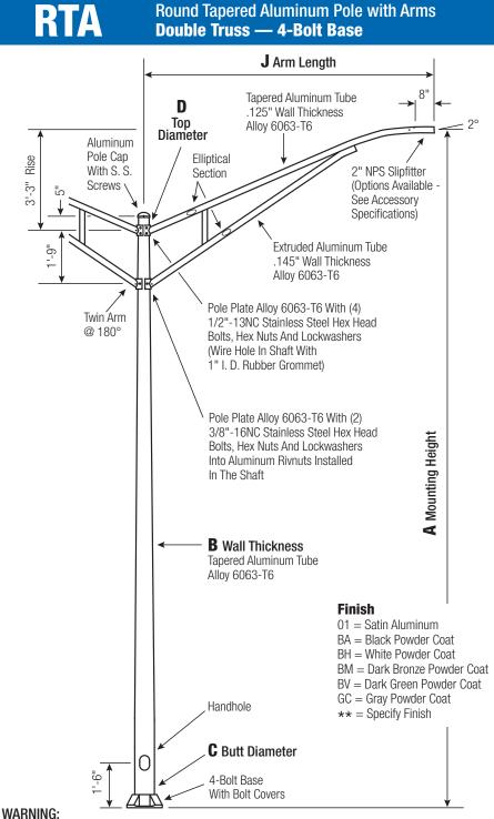
Do not install light pole without luminaire.
