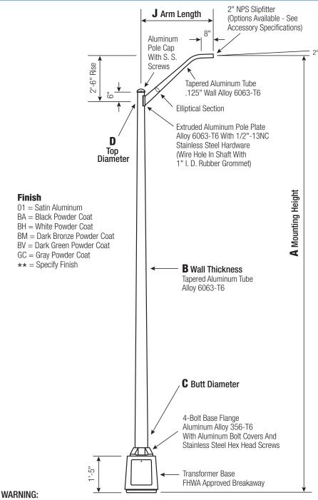
Do not install light pole without luminaire.
